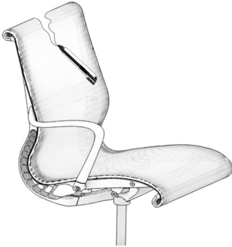
11.1. Using a Utility Knife cut Seat Fabric in half.
