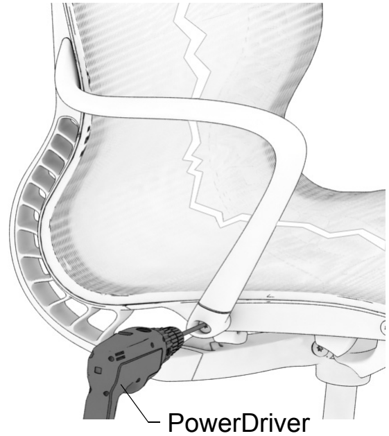
12.1. Using a PowerDriver with a T-27 bit, remove Shoulder Bolt.
