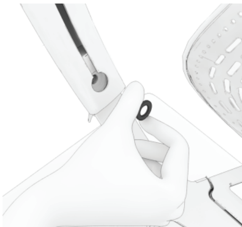
11. Remove the washer from arm. New Arm Support Post does not use washer.
