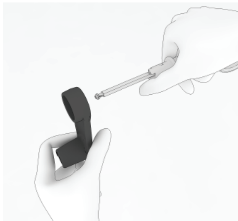
41. Insert new front link into tilt limit control.
