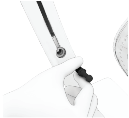
10. Arm Support Post removed.
