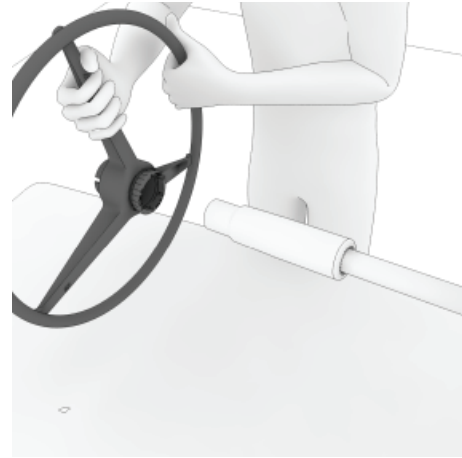
4. Remove footring from the cylinder.
