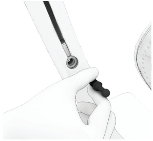
10. Arm Support Post removed.
