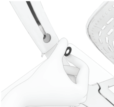
11. Remove the washer from the arm. New Arm Support Post does not use washer.
