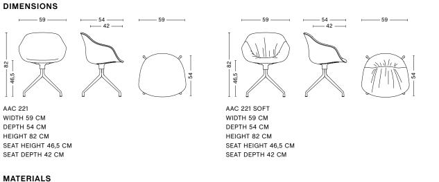
SHELL Injection molded solid-colored polypropylene shell with armrest. Made from 100% post-consumer recycled PP.
